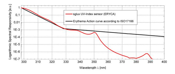
Radiometer for risk assessment of solar UV radiation according to ISO 17166
